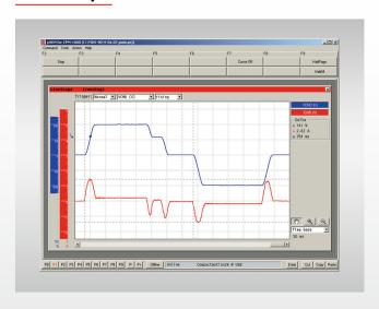
Drive calibration is facilitated by the real-time debugger's Live Scope, which allows observation and analysis of the drive's response characteristics at the computer. One of Live Scope's special features is to display in real-time mode like an oscilloscope, which allows immediate observation of events in the drive system.
